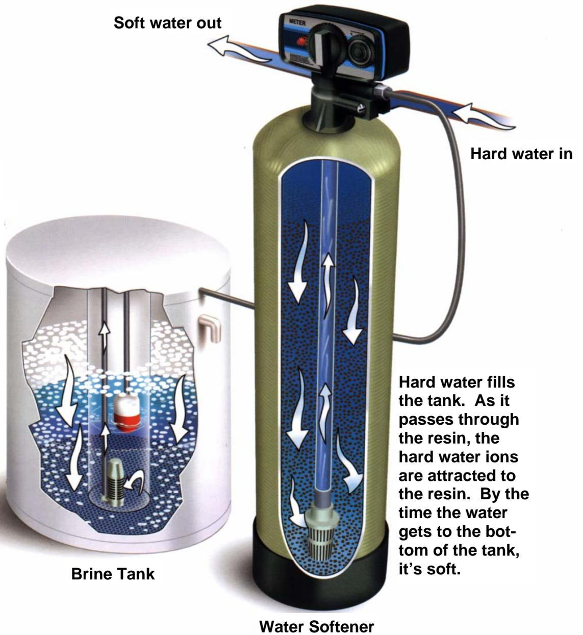
Hard water fills the tank. As it passes through the resin, the hard water ions are attracted to the resin. By the time the water gets to the bottom of the tank, it's soft.
